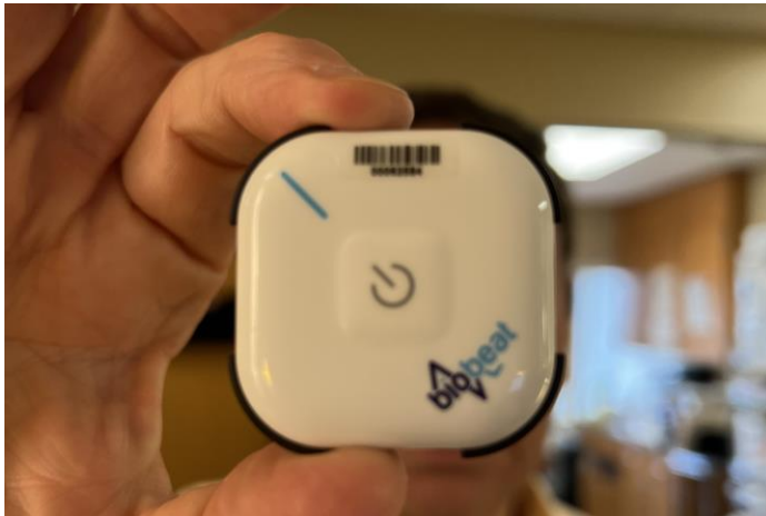
The new Biobeat 24-hour ambulatory blood pressure monitor (ABPM) accurately measures blood pressures without needing an arm cuff, so it is much more comfortable than previous 24-hour devices.
